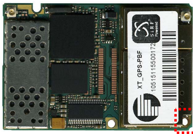
Figure 52: Mounting holes on XT55/56
