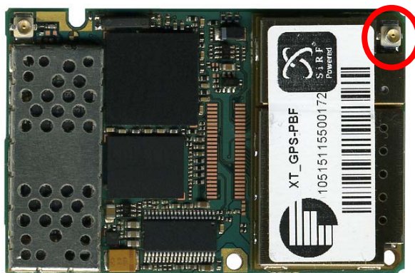
Figure 35: GPS antenna connector (U.FL-R-SMT connector)
